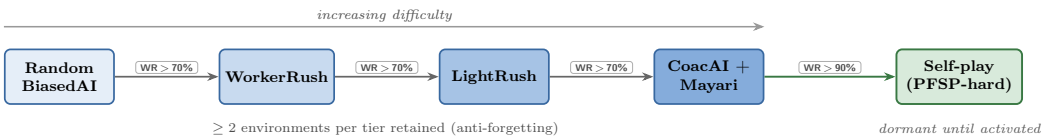
Figure 9.5: Automated opponent curriculum. Each bot environment is promoted to the next tier once its sliding-window win rate exceeds 70%, with at least two environments per tier kept to prevent forgetting. Self-play stays dormant until every terminal-tier opponent is mastered, then switches to PFSP-hard sampling against historical checkpoints.
